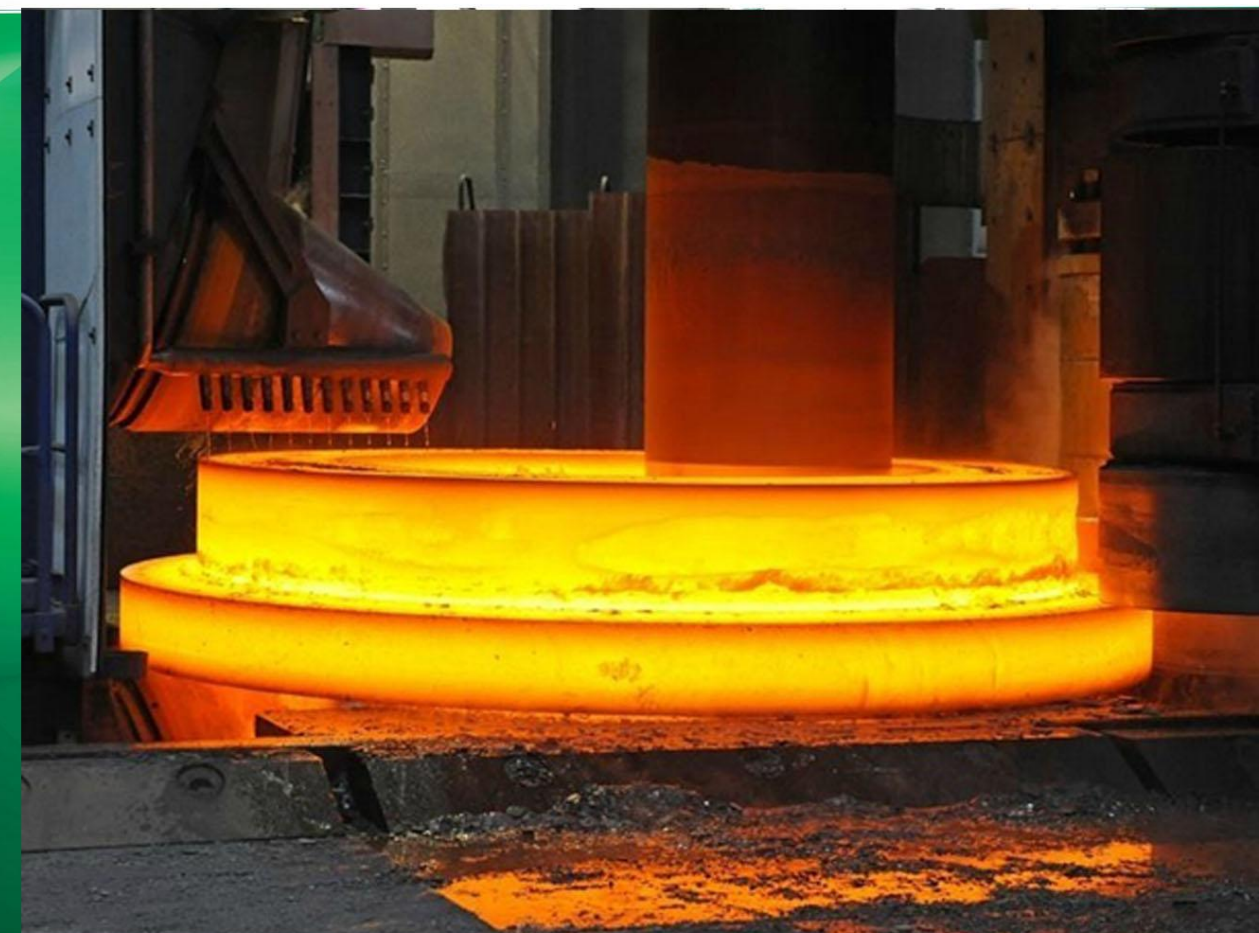
数控径碾环机生产线 CNC ring rolling machine production line
